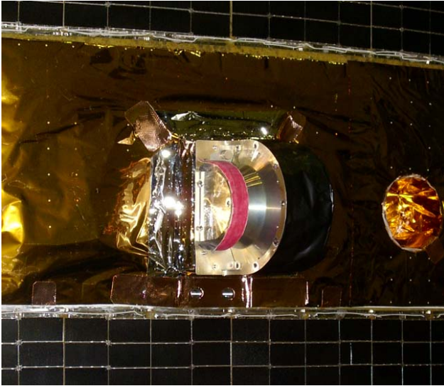
Fig. 8. Photograph of TC-2 PEACE Sensor head showing arrangement of electrostatic conductive materials; spacecraft and PEACE thermal blankets and also solar cells above and below the experiment platform. Note the larger collimator of a LEEA sensor vs. the TC-1 HEEA sensor.
