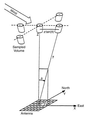
**Fig. 10.** Illustration of the Doppler-beam-swinging (DBS) technique for wind measurements with a five-beam radar. The altitude, range, and zenith angle are denoted by z, r, and  $\theta$ , respectively
