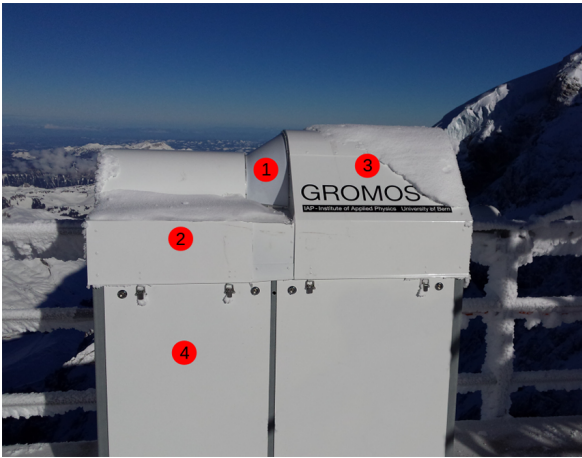
Figure 2. GROMOS-C at the terrace of Sphinx during the Jungfrau-joch campaign (1: Teflon window, 2: Microwave receiver, 3: Calibration targets, 4: Computer and spectrometer).
