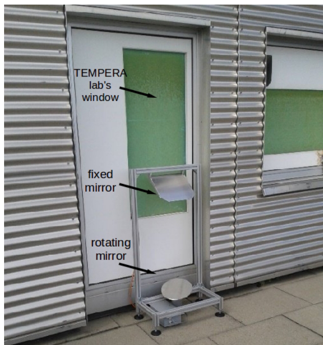
Figure 3. Secondary mirror installed on the roof of the ExWi building at the University of Bern.
