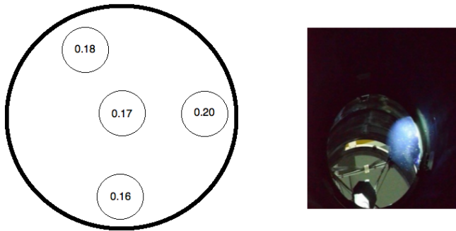
Figure 5. Left: representation scheme of the R_{tf} values in functions of the illuminated portions of the RMR-H 2 O telescope surface. Right: example of the partial illumination of the mirror by the optical arrangement of the calibration lamp.
