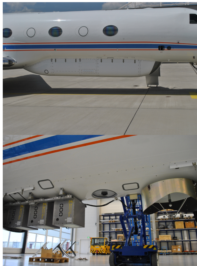
Figure 1. Top: closed belly pod mounted on HALO. Bottom: remote sensing instruments underneath the body of HALO (from left to right: HALO-G, HALO-KV, and HALO-WF module; lidar window; and cloud radar MIRA-36 antenna).
