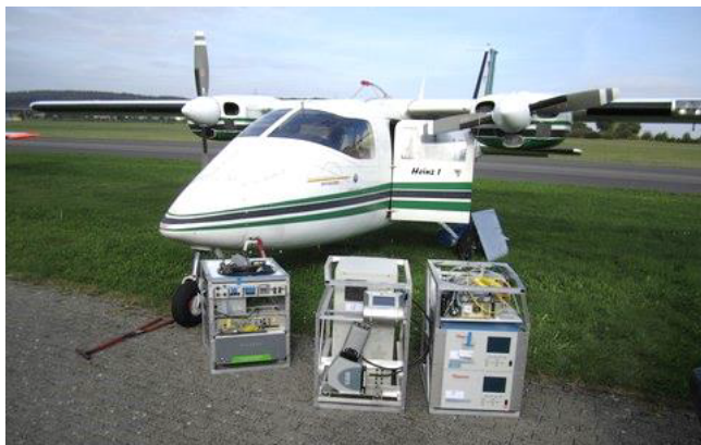
Figure 3. Instruments, mounted in racks, for ready installation in the Partenavia P68B airplane behind. The particle inlet can be seen on top of the fuselage (picture taken by B. Schneider, enviscope GmbH).
