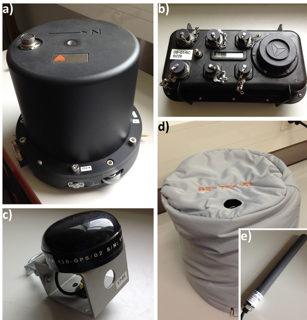
Figure 2. Equipment used for the installations described in this manuscript. (a) Reftek 151 60 s sensor, (b) Reftek 130/130S digitizer, (c) Reftek 130 GPS antenna, (d) textile thermal insulation cover for the sensor, (e) mobile network antenna.
