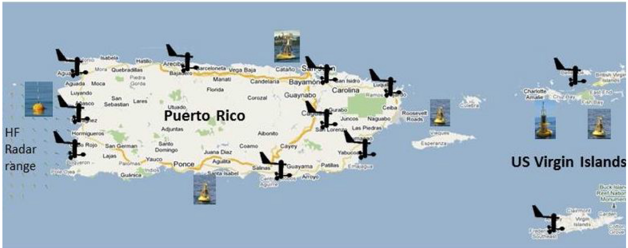
Fig. 7. CariCOOS weather stations and buoys, Puerto Rico and USVI. In the USVI the two anemometer symbols actually represent a total of six weather stations (map modified from CariCOOS web page, 2012).
