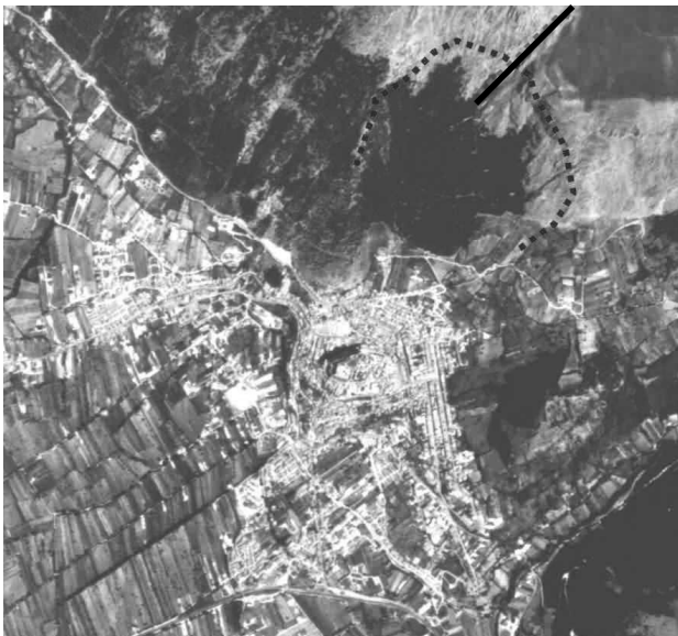
Fig. 1. Aerial photograph of Celano town: are indicated the landslide failure surface (dashed line) and the S. Vittorino fault (solid line).
