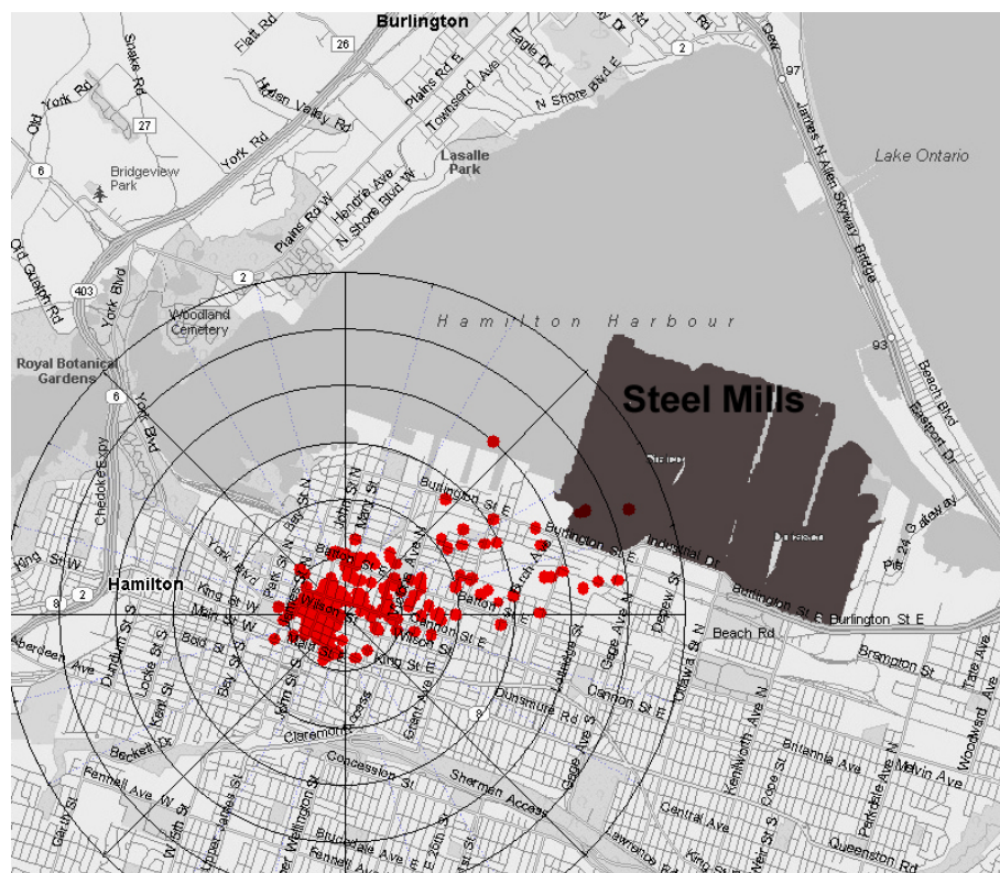
Fig. 7. Polar plot for the local anthropogenic emission factor scores (1999 data) superimposed on a street map of the city Hamilton (map source: http://mappoint.msn.com ). Each radial increment represents the relative magnitude of the absolute factor scores. The measuring site is represented by the center of the polar plot. The dark grey area indicates the two large steel mills in Hamilton.
