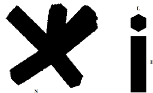
Figure A6. Schematic description of hydrometeor shapes for subsequent simulations of bullet rosettes.
