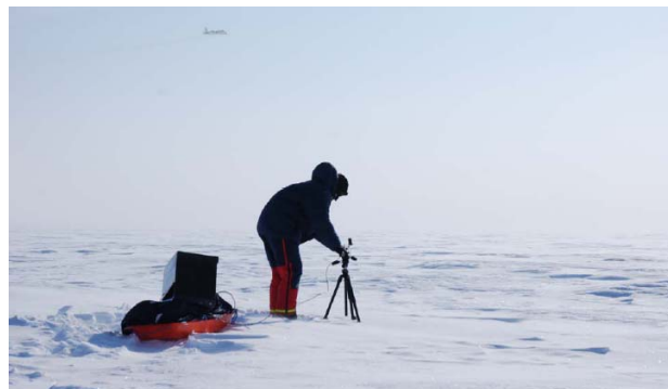
Fig. 1. Spectral albedo measurements on Elson Lagoon on 15 April 2008, with the P-3B airplane in the background. The leveled cosine collector is rotated to collect light from upward and downward hemispheres sequentially. The light is carried through a fiber-optic guide to the ASD spectral radiometer and its computer, which are mounted on the sled.
