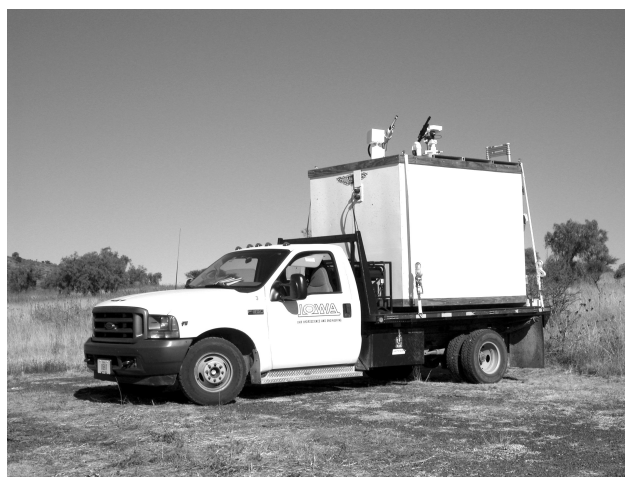
Fig. 1. The University of Iowa mobile vertical lidar (1064 nm 50 Hz 25 mJ/pulse laser, 100 MHz digitizer, 1.5 m spatial and 1 s temporal resolution) during the MILAGRO 2006 campaign.
