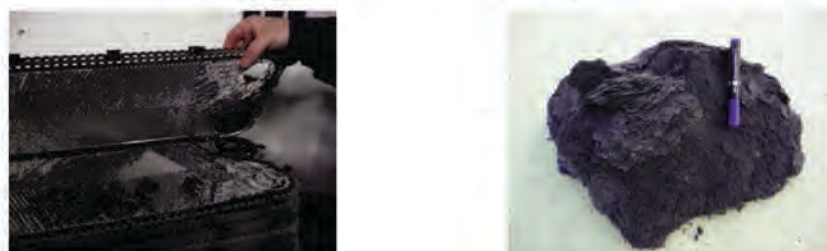
Figure 1: Precipitation of elemental sulphur on plate heat exchangers (left). Massive scalings of Mg-calcite at a heat exchanger (right).
