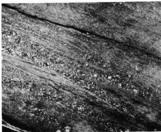
Fig. 5: Disseminated pyritic ore in thinly banded quartzitic-chloritic ganguematerial. Locality: Schwarzwand/Grossarlal handspecimen, magnified; lower side = 3 cm.
