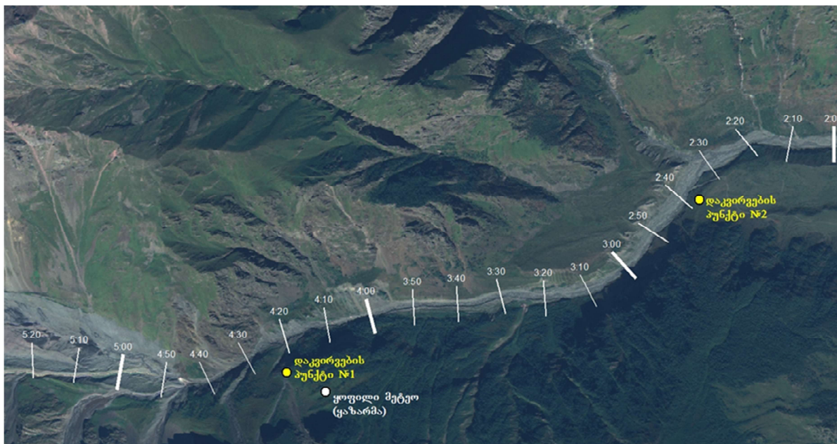
Fig. 4: Map: Warning Times (Min/Sec), Observation points (left/right point at 2.284m and at Amali/Devdoraki confluence (1.715m) and Warning and Communication point (right).
