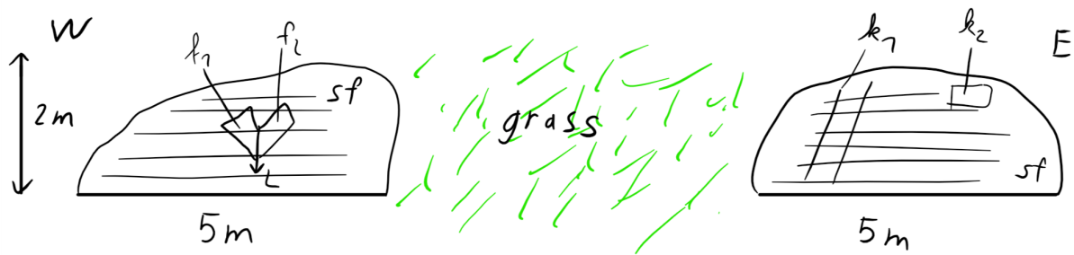
Figure 19: Sketch of outcrop 7. Abbreviations: f = fault, k = joint, L = Lineation, sf = schistosity
