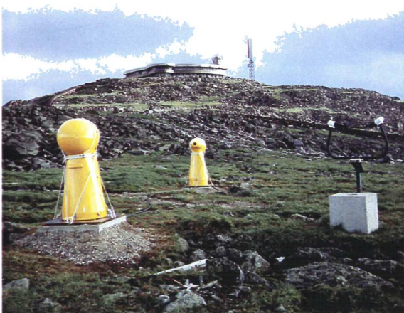
Different techniques for measuring visibility have been tested in very dense fog at the Observatory: data from both the two transmissometers on the left and the scatterometer on the right were compared to human visibility measurements in this study (source MWO Archives)
