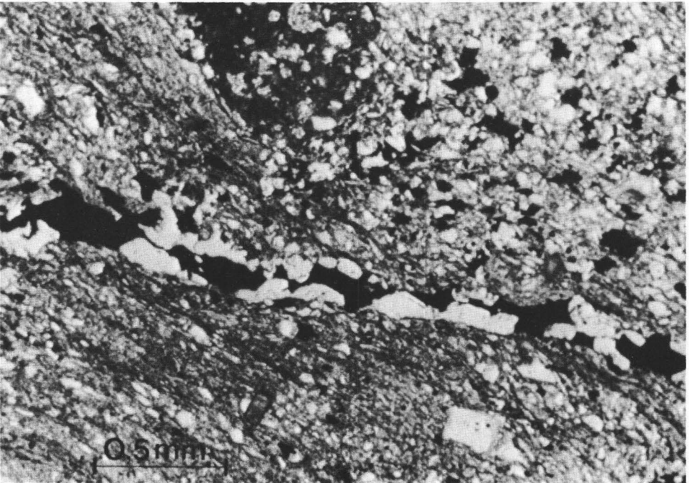
Fig. 8. Albite-chalcopyrite veinlet cutting the mineralized siltstone. Transmitted polarized light.
