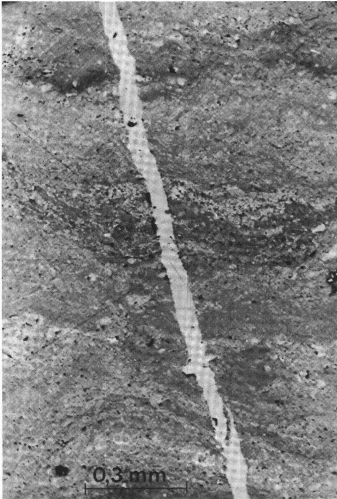
Fig. 10. Cinnabar veinlet cuts "stell ore" showing bedded structure. Reflected polarized light.
