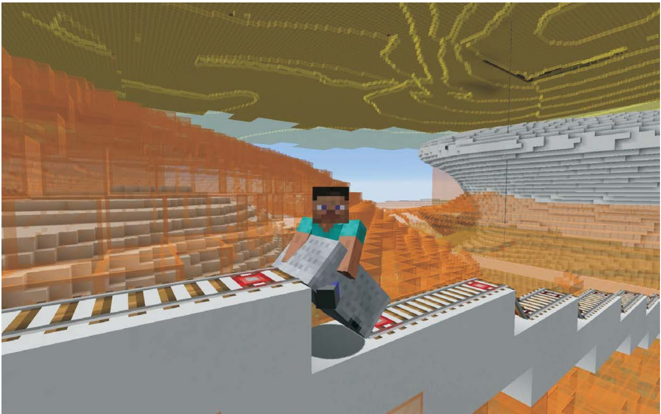
Figure 17. Rollercoaster ride around a salt structure in the German North Sea realized in Minecraft®. The solid grayish body in the background on the right represents the salt structure; geologic base horizons are realized in colored glass (yellow: Quaternary, orange: Tertiary). The vertical line in the background symbolizes an exploration well. The model is also available in VR.
