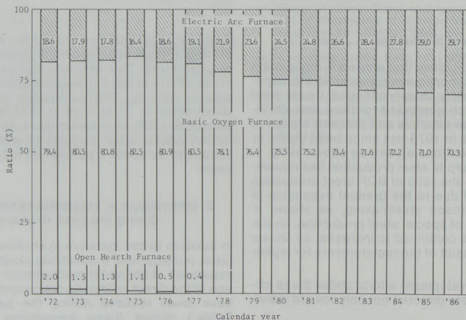
Fig. 2 Trends in ratio of basic oxygen furnace steel in Japan
