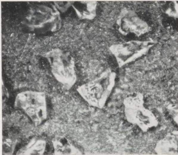
$\text{Al}_2\text{O}_3$  BKR 46 (420 ... 350  $\mu\text{m}$ )
