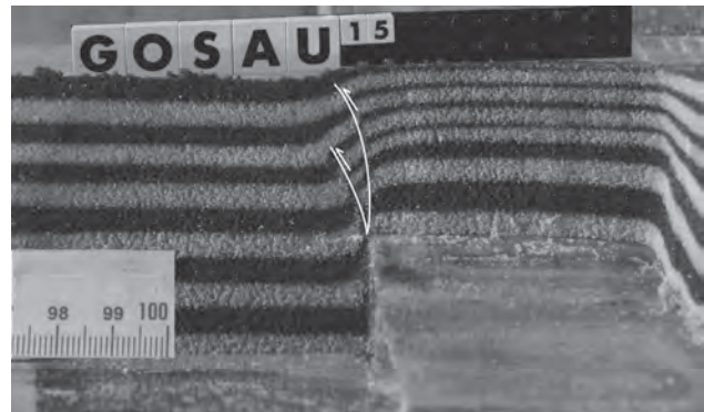
Fig. 2: Crosscut perpendicular to the tear fault within the analogue model showing two steep thrusts.
