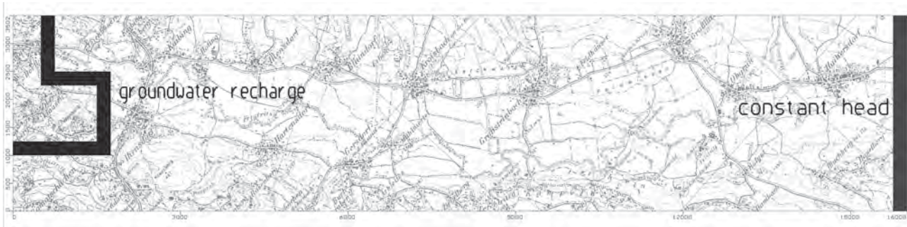
Fig. 7: Boundary conditions in the lower model layer.
