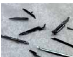
Figure 1. Single crystals of off-stoichiometric \text{Cu}\square\text{GaGeS}_4 (left) and \text{Cu}\square\text{GaSnS}_4 (right).
