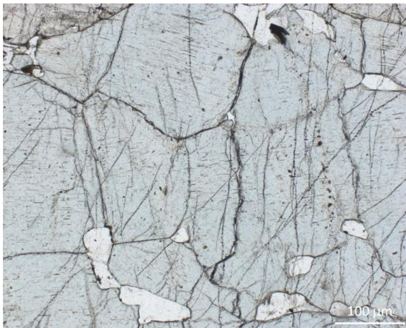
Figure 1. Apatite with needles of oriented triphylite (under plane-polarized light).
