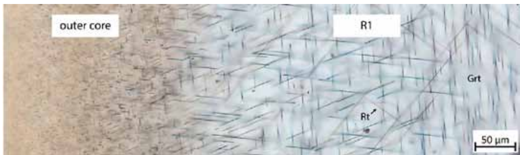
Figure 1. Optical micrograph (plane polarized light) of the microstructural transition from the outer garnet core to the garnet growth zone R1 in a \{112\} Grt growth sector. Note the increasing aspect ratio of rutile (Rt) inclusions and the decrease in garnet (Grt) colour intensity from the outer core to R1.
