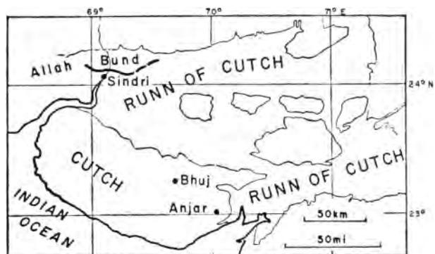
FIGURE 24: The position of the Allahbund that formed during the devastating earthquake of 16 th June 1819 and led to the total submergence of the Fort of Sindree, except for one tower (from Richter, 1958, fig. 31-9).
