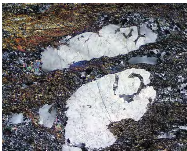
FIGURE 6: Photomicrograph of embayed quartz as a indicator of a shallow intrusion depth of the protolith of the KG (sample A-34, X Nichols, magnification 10x).
