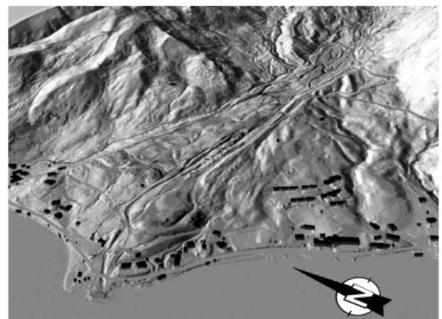
FIGURE 4: 3D view of the Gschlifegraben landslide (analytical hillshading, ALS, slant view from SW).
