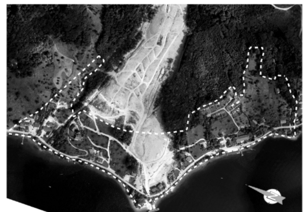
FIGURE 2: Hazard zone map, officially approved in 1987. At its periphery, the hazard zone ("red zone") is wider than 950m.
