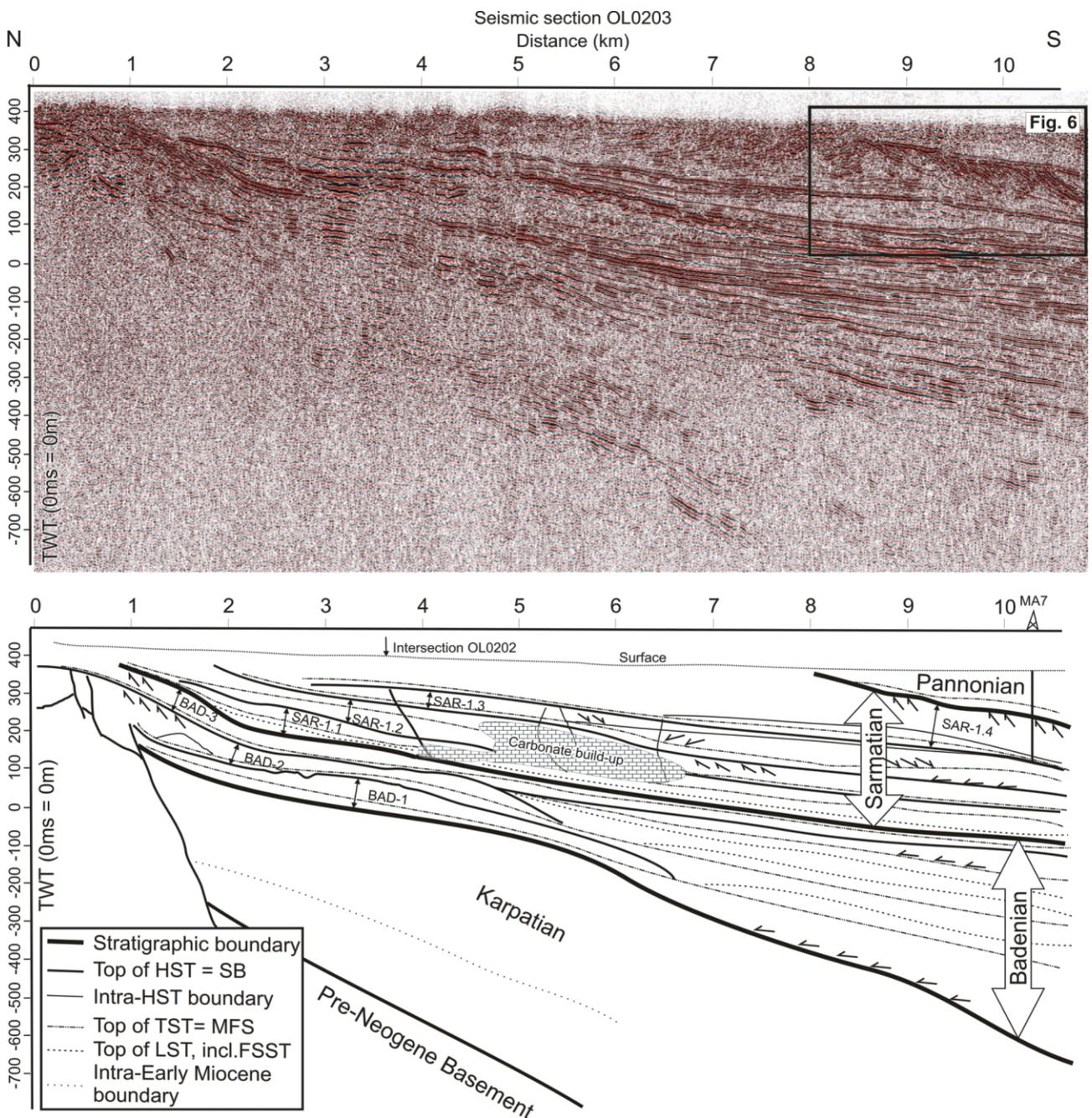
FIGURE 3: N-S seismic section OL0203 in the Upper Lafnitz Valley and its interpretation. See Figure 1 for location of seismic section.
