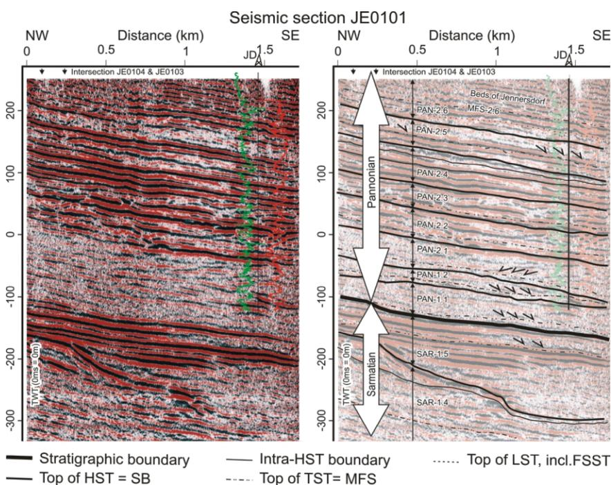
**FIGURE 15:** Seismic section JE0101 with gamma (γ) and resistivity (R) logs of well JD and its interpretation. See Figure 1 for position of seismic section.
