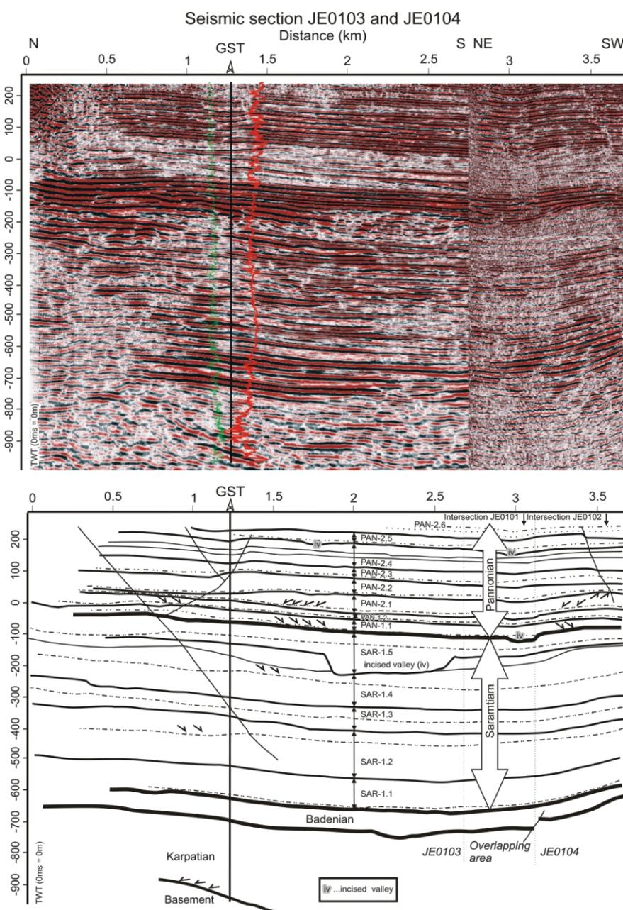
**FIGURE 17:** Seismic sections JE0103/JE0104 with gamma ( $\gamma$ ) and resistivity (R) logs of well GST and their interpretation. See Figure 1 for position of seismic sections and Figure 15 for legend.
