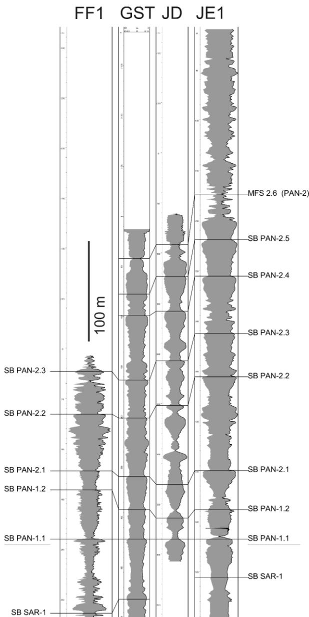
**FIGURE 1B:** Cross section based on mirrored resistivity logs of wells Fürstenfeld 1 (FF1), Grieselstein Thermal1 (GST), Jennersdorf (JD) and Jennersdorf1 (JE1) showing the subdivision of the Pannonian succession into 4<sup>th</sup> order sequences. The MFS-2.6 corresponds to the MFS-2 of PAN-2 after Sacchi and Horváth (2002). Datum is SB PAN-1.1.
