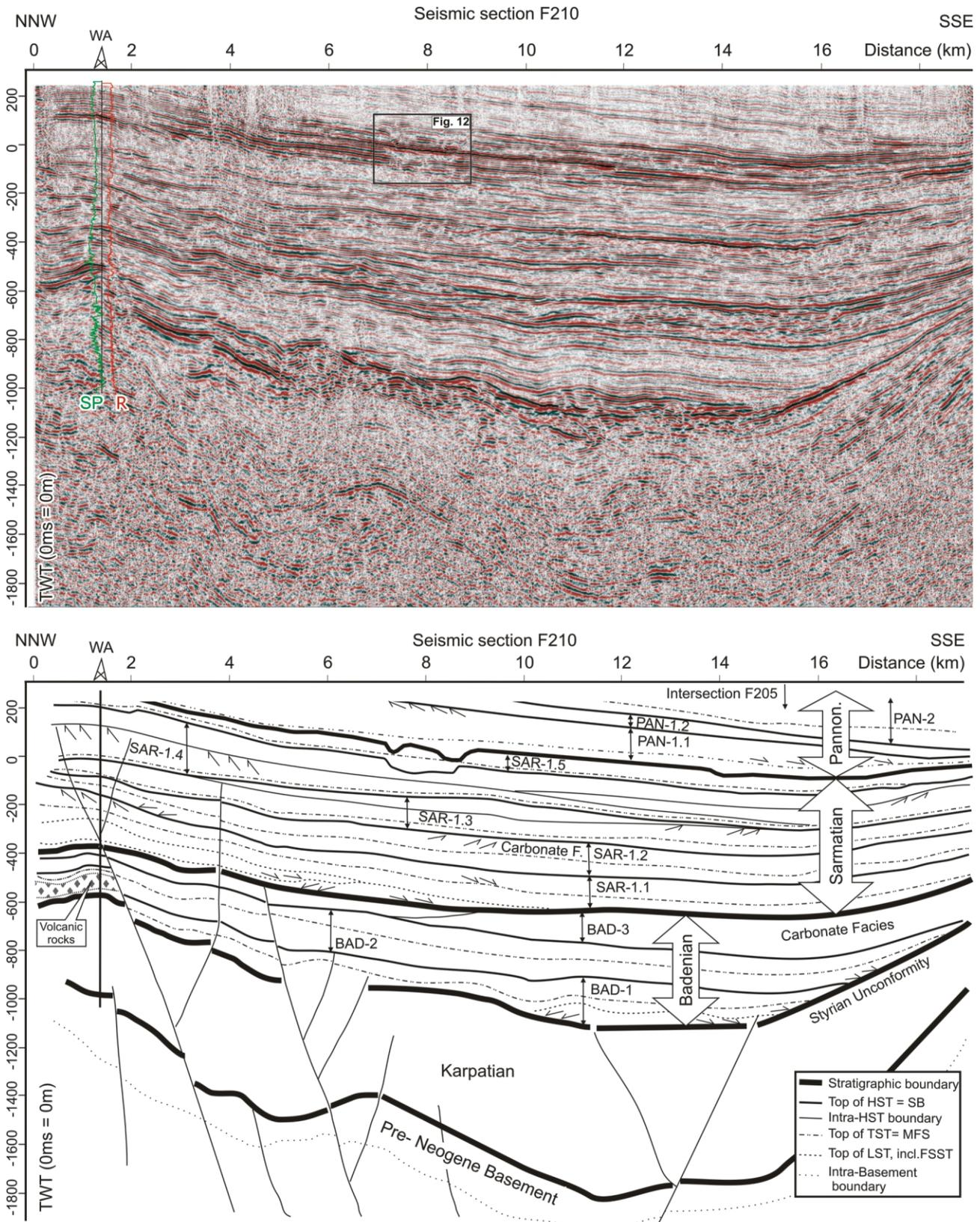
**FIGURE 7:** Seismic section F210 with Spontaneous Potential (SP) and resistivity (R) logs of well Walkersdorf 1 (WA) and its interpretation. See Figure 1 for position of seismic section.
