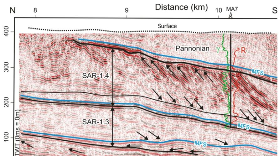
**FIGURE 6:** Detail of southern part of seismic section OL0203 showing southward progradation of an Upper Sarmatian (SAR-1.4) delta. Gamma ( $\gamma$ ) and resistivity (R) logs of well MA7 are displayed. For position see Figure 3.
