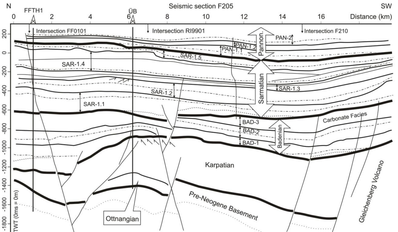
**FIGURE 8:** Seismic section F205 with gamma (γ) and resistivity (R) logs of wells FFTh1 and Spontaneous Potential (SP) and resistivity (R) logs of Übersbach 1 (ÜB) and its interpretation. See Figure 1 for position of seismic section and Figure 7 for legend.
