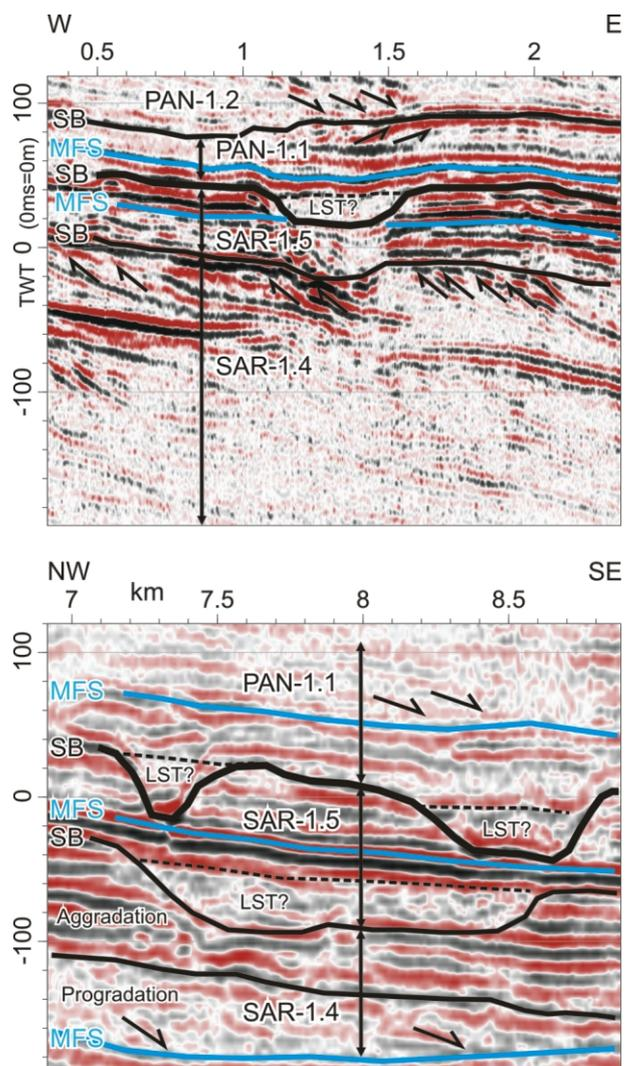
**FIGURE 12:** Details of seismic sections RI9901 (Figure 10) and F210 (Figure 7) showing erosion events at the top of SAR-1.4 and top of SAR-1.5 (= Sarmatian-Pannonian boundary).
