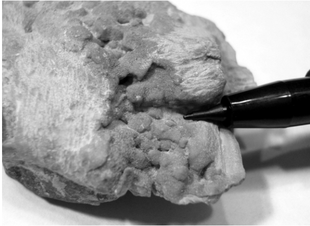
FIGURE 5: Sample of conglomerate of Gamperdona valley. At the sampling location (cf. Fig. 2), conglomerates contain levels of openwork fabric, and are lithified by isopachous fringes of calcite cement. Pen tip for scale.
