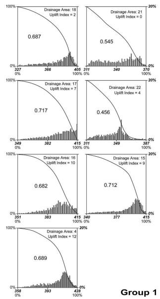
FIGURE 6A: Hypsometric curve and topographic distribution (columns) of 5th-order basins, Group1 (for grouping criteria see explanations in the text). For every basin the uplift index is given in the upper right.
