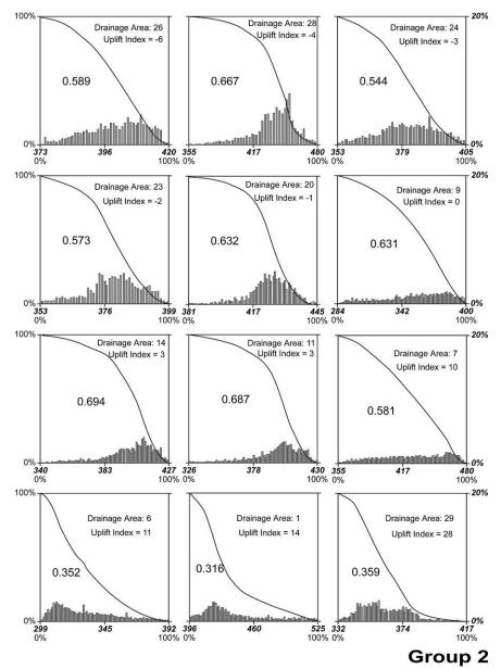
FIGURE 6B: Hypsometric curve and topographic distribution (columns) of 5th-order basins, Group2 (for grouping criteria see explanations in the text). For every basin the uplift index is given in the upper right.
