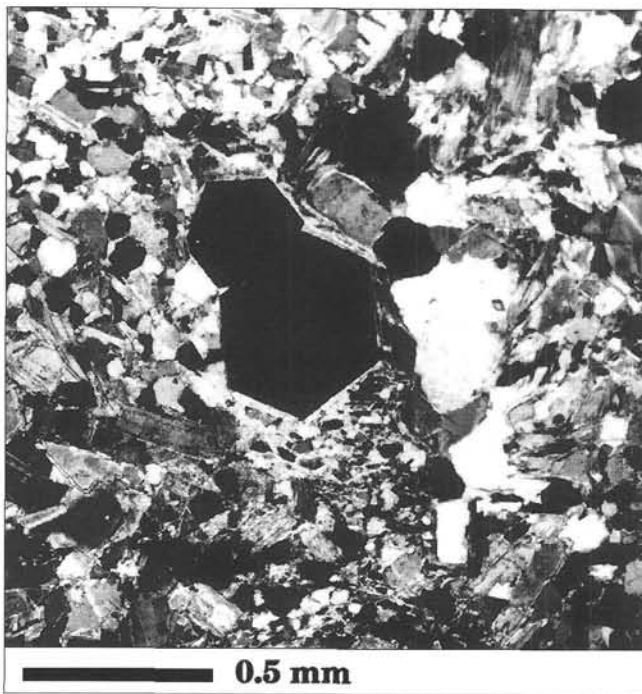
Text-Fig. 4. Idioblastic garnets with no resorption and decompression reaction signs demonstrate static periplutonic growth and are represented by the linear size distribution (population density versus crystal size). Sample M.K. 17. Cross-polarized light.
