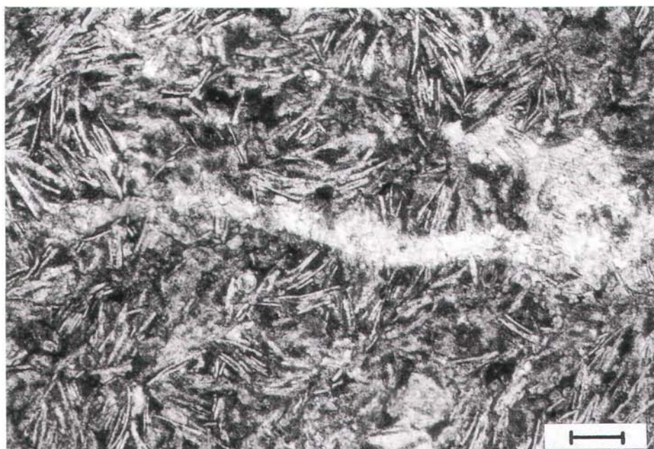
Fig. 148: Thin section photomicrograph of filament packstone (Dogger). Position 5 in Fig. 135. Kritsch quarry; length of scale = 0.25 mm.
