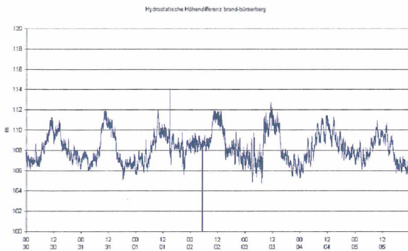
Fig. 13: Hydrostatic height difference Bürserberg-Brand, August 30 – September 6, 1999, a week with well pronounced valley winds
