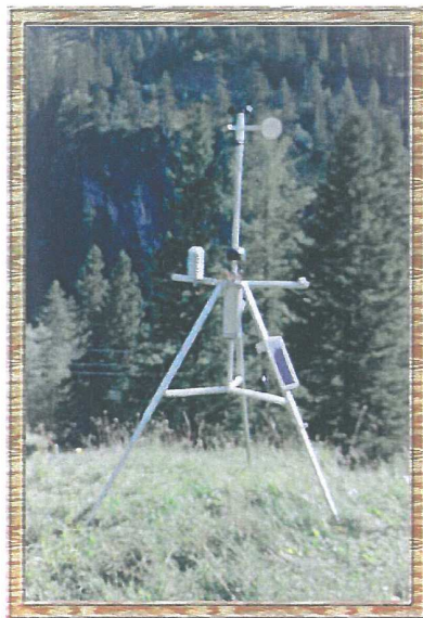
Fig. 15: Station Schattenlagant. The pressure sensor is situated in the tube at the upper part of the tripod. Depending the orientation of the solar panel with regard to the foehn wind direction, the sensor may be in the lee of the solar panel or hardly influenced.
