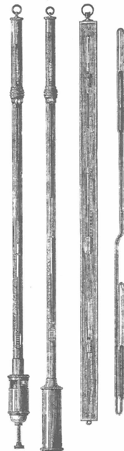
Fig. 4.13. Four barometers in common use in the Austrian network. From left to right: one Fortin-, one Kew- and two siphon barometers
