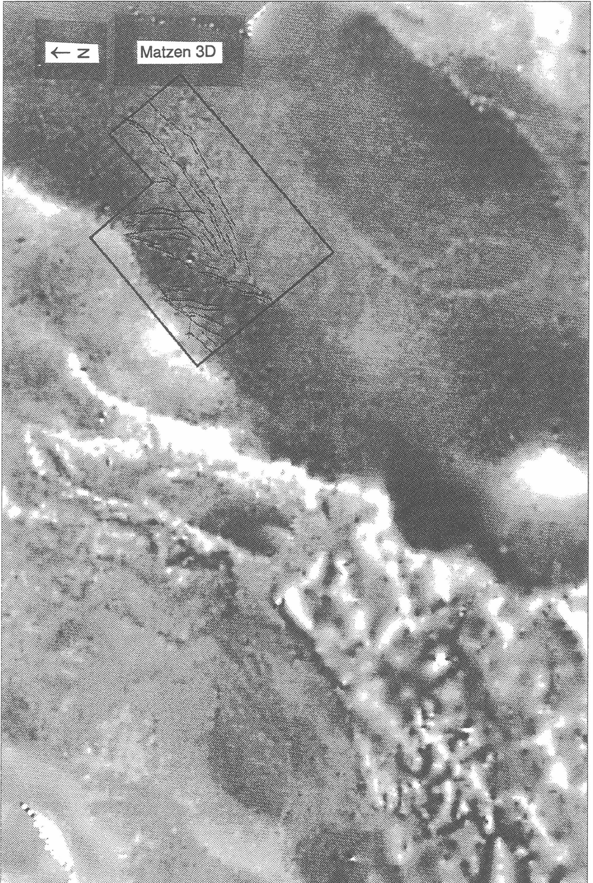
Figure 4: Vertical gradient map in the Matzen area with overposted seismic faultcuts of the near top Sarmat horizon.
