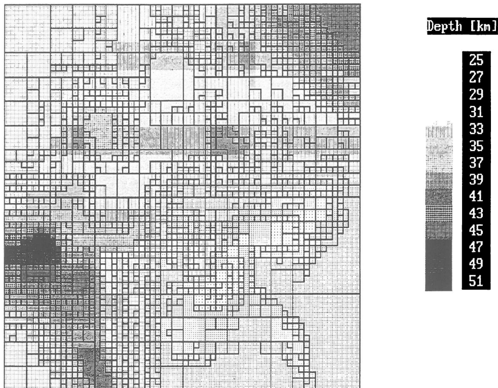
Figure 2. Horizontal arrangement of the prism system of the model of the upper mantle in Central Europe. Depth values refer to the upper side of the prisms.
