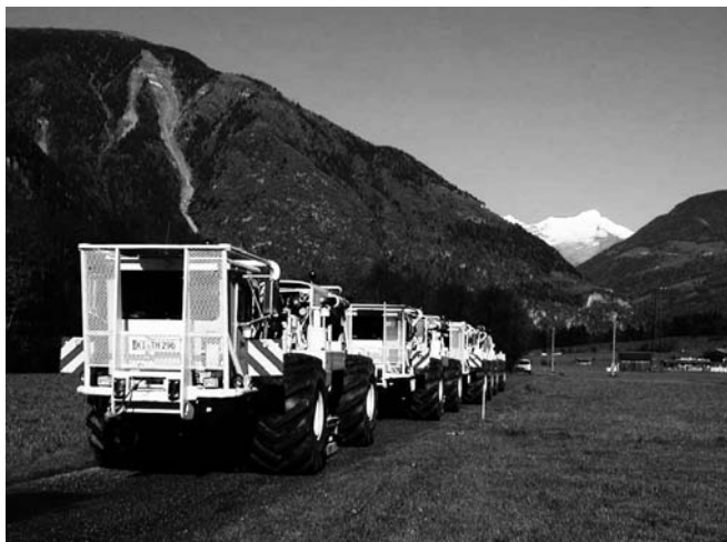
Figure 1 Vibrators in operation in the Zillertal.
