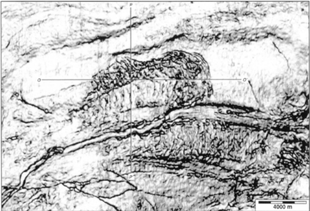
Fig. 43: A coherency slice (map view) at 144 milliseconds below the seafloor illuminates the slump in much greater detail than the vertical sections in Figure 42 (reproduced with permission of BP).
