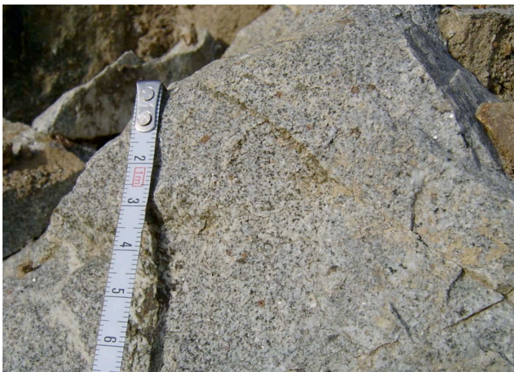
Figure 23 Plagiogranite in the Tóbérc quarry. 2-4 mm big reddish brown garnet is common in samples collected close to the border towards the gabbro.
