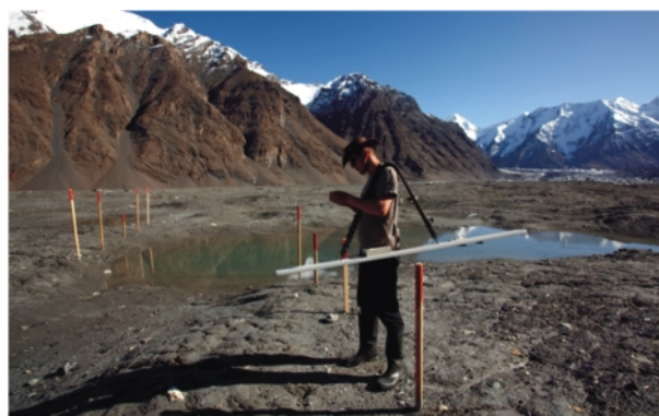
FIGURE 8: FDEM-measurements in the Peremitschka test site cross water-filled depressions (photo courtesy of Marc Roussel, 24 August 2009).
