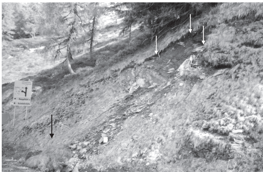
Fig. 5: A shallow translational slide on the upslope edge of a human-modified ski-run in the Hauser Kaibling ski-area. Note the ~20 cm long field book for scale in the centre. The white arrows indicate the area of release. The underlying bedrock material (schist) is visible. The black error indicates the landslide deposits (KELLERER-PIRKLBAUER 2001).
