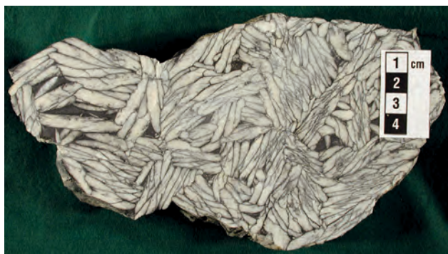
Fig. 10: "Pinolitic" texture of the magnesite from the Hohentauern deposit
