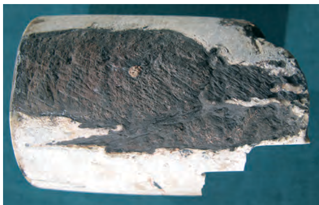
Fig. 4/5: Oxidic manganese ore infilling in the dissolution holes of the Kardosrét Limestone in core of a borehole drilled on the western side of the strike-slip fault of the long trench.
