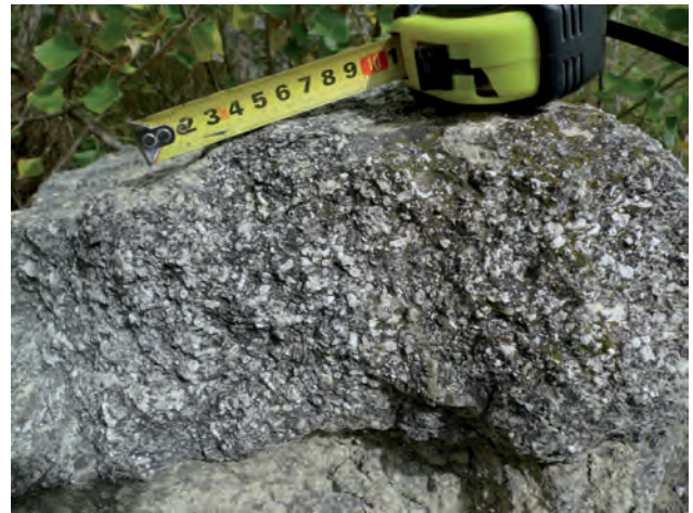
Fig. 14: Detail of the coralgall limestone (Leithakalk) from the upper part of the Sandberg quarry.
