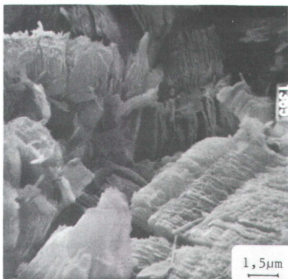
Tvoříhráz deposit, 1.1.3. Fig. 5: Aggregates of tubular halloysite and single plates of kaolinite (kaolin F).
