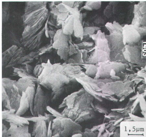
Jimlikov deposit, 1.1.1. Fig. 6: The microfabric indicates irregular distribution of predominating single plates together with some aggregates of kaolinite (rounded and thickened rims are characteristic similar to the Osmosa samples, see Fig. 1) (kaolin B).
