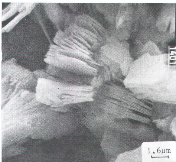
Fig. 5: Stacks of kaolinite with idiomorphic pseudo-hexagonal crystals (parent granite).
