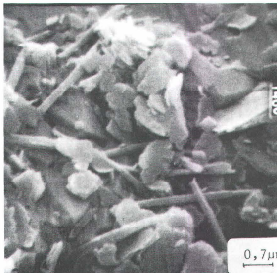
Hájek (Hroznětín) deposit, 1.1.1. Fig. 4: Secondary components of tubular halloysite beside flakes of platy kaolinites (kaolin E).
