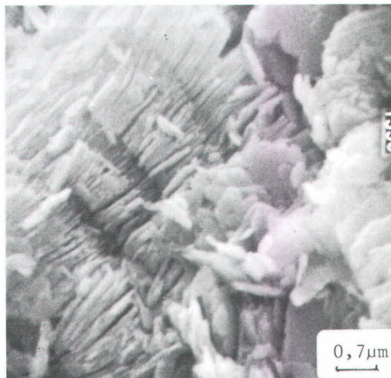
Otovice (Katzenholz) deposit, 1.1.1. Fig. 2: Book-like aggregates with rounded single plates of kaolinite (kaolin D).
