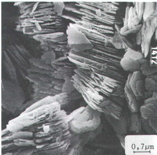
Fig. 3: Stacks of idiomorphic pseudo-hexagonal kaolinite plates (siltstone, "šlika" N).
