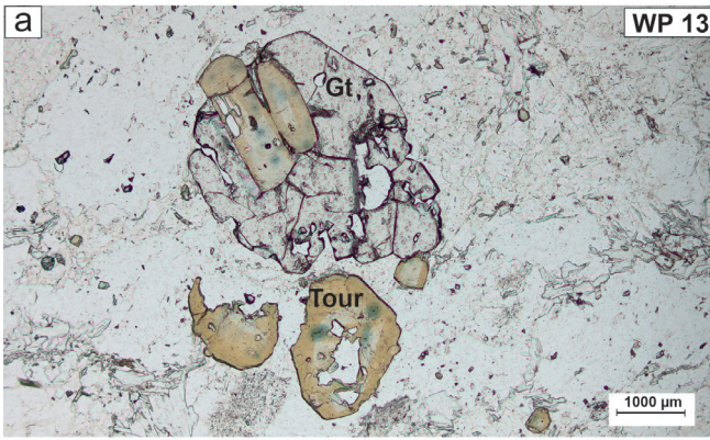
Text-Fig. 2. a) Coexisting garnet and tourmaline. Tourmaline with pleochroic halos (blueish colour) around the zircon inclusions. b) Zoned tourmaline with homogeneous core also with pleochroic halos around zircons.
