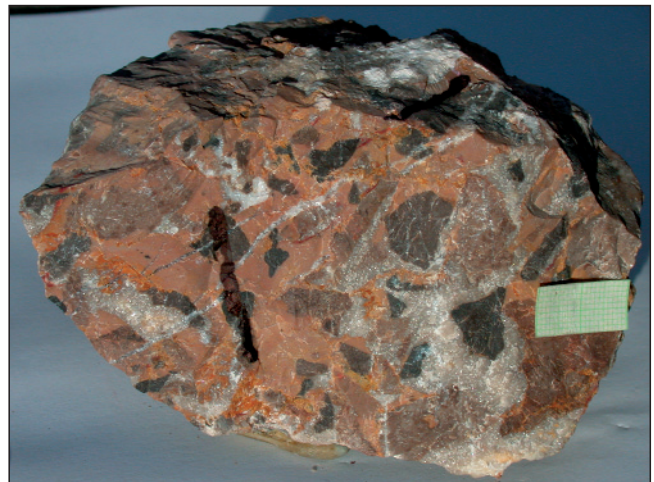
Text-Fig. 11. Brown and black clasts in a tan mudstone matrix with solution cavities filled by sparry calcite.
